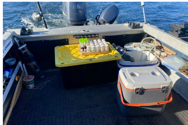
Photo 2. An image of all of the required sampling gear and bottles, including: CTD and backup rod, cooler for putting samples in to keep them cool after collection, all sample bottles (phytoplankton, nutrients, chlorophyll bottles), except biotoxin bottles, Niskin bottle and Secchi disk. Photo credit: Nicole Frederickson
