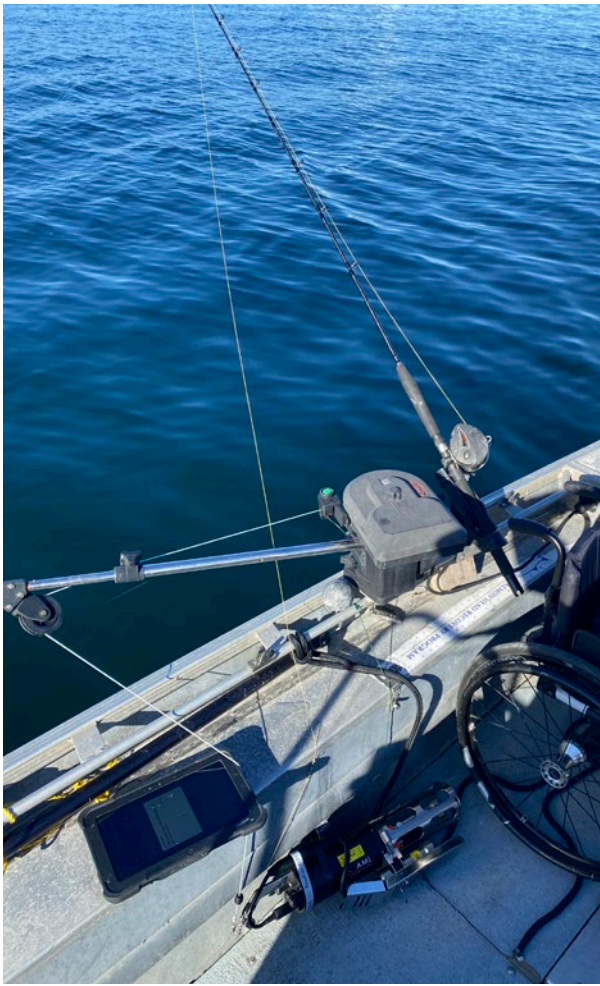
Photo 5. An image showing the CTD connected to the downrigger cable and the back-up safety line (heavy duty Penn fishing rod and reel, with 80 lb test braided fishing line).
