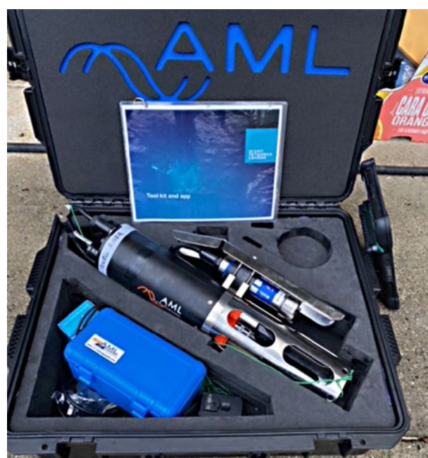
Photo 4. An image of the AML CTD instrument used to collect conductivity, temperature, dissolved oxygen and depth measurements. Photo credit: Nicole Frederickson.
