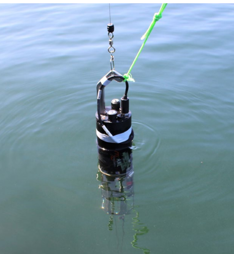
CTD being lowered into the water to measure conductivity, temperature and dissolved oxygen and chlorophyll a. Photo taken by Svetlana Esenkulova.
